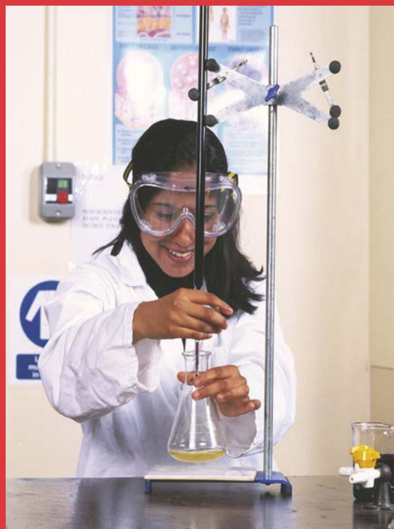
Figure 1.1 A titration is a method used to find the amount of a particular substance in a solution.
